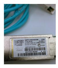
Cisco QSFP-100G-AOC5M 100G QSFP Active Optical Cable, 5-meter
