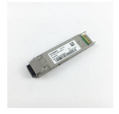
Huawei Optical Transceiver (XFP, 1550nm, 9.95~11.1Gb/s, -1dBm~2dBm, -15dBm, LC, SM, 40km)
