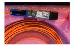
Cisco SFP-10G-AOC7M 10GBASE-AOC SFP+ Cable 7 Meter
