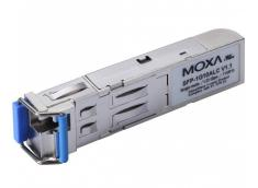
Moxa SFP-1G10ALC WDM-type (BiDi) SFP module with 1 1000BaseSFP port with LC connector for 10 km transmission; TX 1310 nm, RX 1550 nm, 0 to 60°C operating temperature
