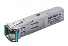
Moxa SFP-1G10BLC WDM-type (BiDi) SFP module with 1 1000BaseSFP port with LC connector for 10 km transmission; TX 1550 nm, RX 1310 nm, 0 to 60°C operating temperature
