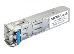
Moxa SFP-1GEZXLC-120 SFP module with 1 1000BaseEZX port with LC connector for 120 km transmission, 0 to 60°C operating temperature
