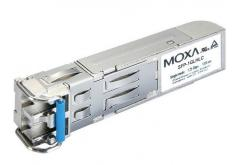
Moxa SFP-1GLHLC SFP module with 1 1000BaseLH port with LC connector for 30 km transmission, 0 to 60°C operating temperature
