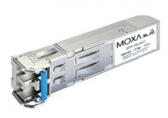
Moxa SFP-1GLXLC SFP module with 1 1000BaseLX port with LC connector for 10 km transmission, 0 to 60°C operating temperature
