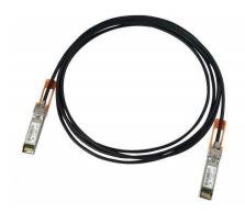
Cisco SFP-H25G-CU5M 25GBASE-CR1 SFP28 Passive Copper Cable, 5-meter
