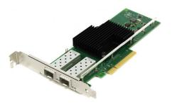
Intel X710 10GbE Dual SFP+ Port Ethernet Converged Network Adapter
