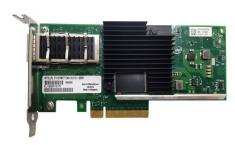
Intel Ethernet Single Port 40GbE QSFP+ Converged Network Adapter
